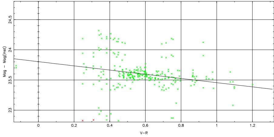
1 parameter fit:  $\text{Mag} - \text{Mag}(\text{Inst}) = 23.66 \pm 0.06 + (-0.11 \pm 0.00) \text{ airmass} + (-0.13 \pm 0.00) \text{ color}$
