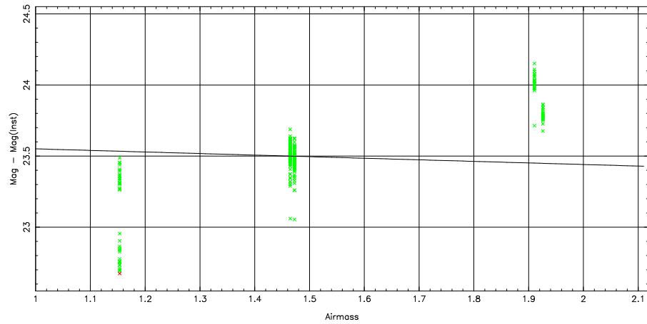
3 parameter fit:  $\text{Mag} - \text{Mag}(\text{Inst}) = 23.66 \pm 0.19 + (0.00 \pm 0.00) \text{ airmass} + (-0.37 \pm 0.32) \text{ color}$
