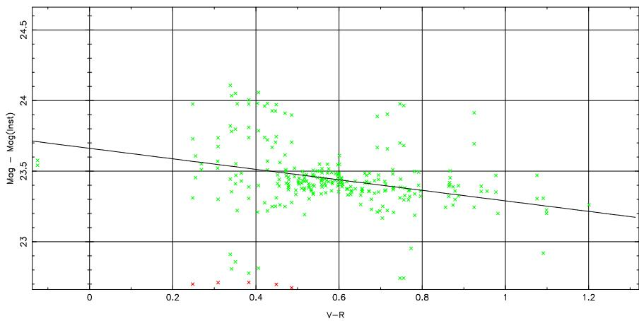
2 parameter fit:  $\text{Mag} - \text{Mag}(\text{Inst}) = 23.80 \pm 0.19 + (-0.11 \pm 0.00) \text{ airmass} + (-0.35 \pm 0.00) \text{ color}$
